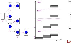
Deployment using a binomial tree Execution time:  $log_2(n) \times 100ms$ For 1000 nodes: 1s without overhead of the engine Gain: Logarithmic factor
