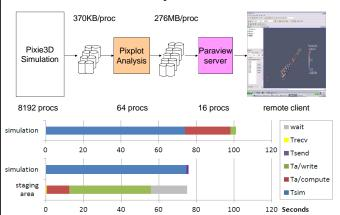
Using 0.78% additional nodes offloading Pixplot and I/O to staging area increases performance by 33% in comparison to inline placement
