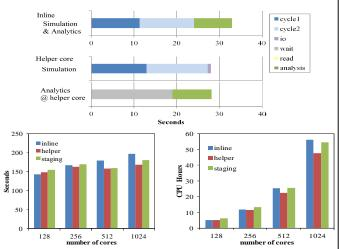
Placing analysis on helper cores in compute nodes achieves the best performance & cost due to spare cycles available there
